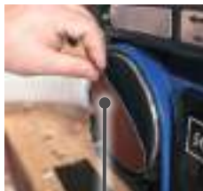
Sanding disc with velcro fastener
