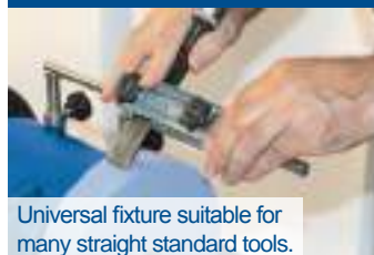
The angle gauge enables quick configuration of the required grinding angle.
