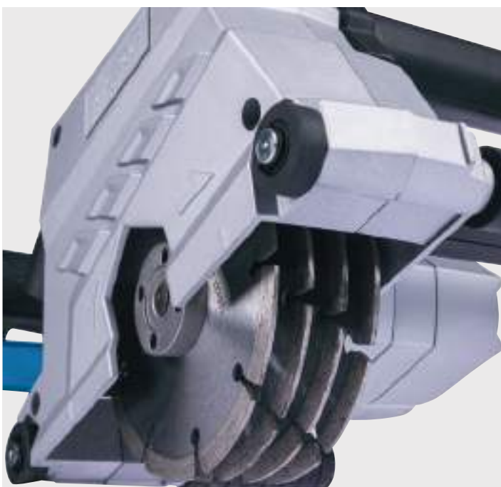
Adaptable cutting width adjustment with up to 4 cutting wheels for narrow and wide chases from 8 to 40 mm.
